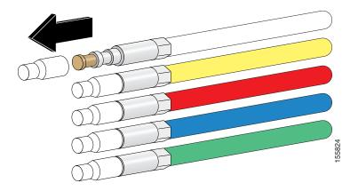
Figure 20 Removing an ESD Cap from an F connector
